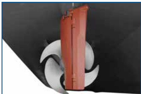
Picture 1: Becker Flap Rudder Twisted (© Becker Marine Systems)
