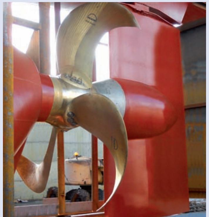
Playa de Ris for PEVASA with 14 m 2 twisted rudder with integrated bulb
